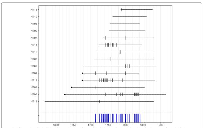
**Fig. 3** Fire-history chart for the Nichols Preserve in the piedmont of North Carolina. Horizontal lines show the time series of an individual tree. Vertical tick marks on the horizontal lines represent fire scars. The composite fire-scar series at the bottom of the figure displays all fire events through time. This figure was generated in the R package *burnr* (Malevich et al. 2018). Data were collected in 2019–2021
