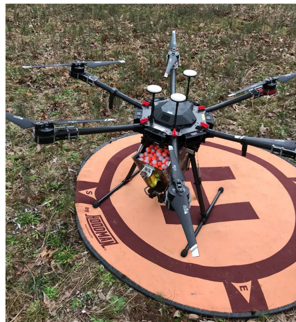
Fig. 1 DJI Matrice 600 Pro drone with attached hopper filled with dragon eggs. (Photo credit: Dr. Callie Schweitzer)
