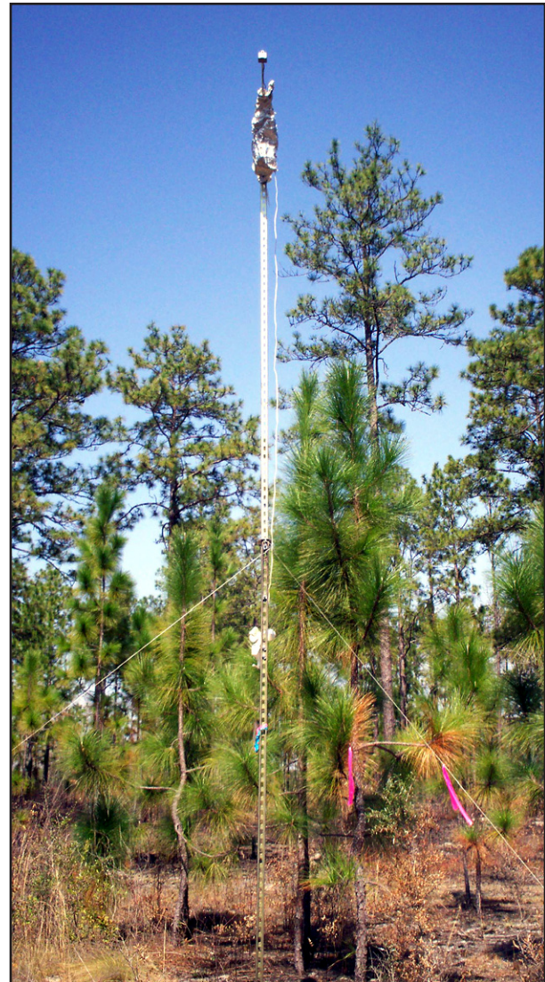
Figure 2. Overhead fire monitoring station for field use consisting of a downward-pointing dual-band infrared sensor, weather and gas (CO, CO 2 ) sensors, all mounted on a portable 6.2 m tower. The image was captured during a series of experiments (Rx-CADRE) conducted in the longleaf pine-wiregrass ecosystem of the southeastern United States.
