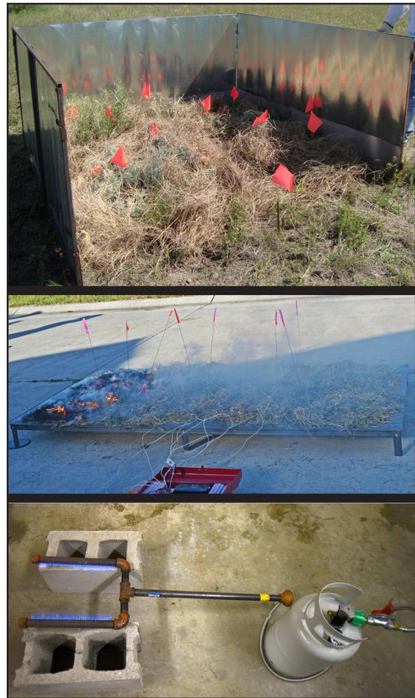
**Figure 1.** Images for each of the three experimental approaches conducted in Montana and North Dakota, USA, from 2012 to 2014. The top panel shows the burn box with one missing sheet to show the placement of the added biomass with *in situ* vegetation. The middle panel shows the burn table using plants rooted in pots and added timothy hay. The bottom panel shows the propane prong that was used inside an enclosed structure to burn plants rooted in pots.
