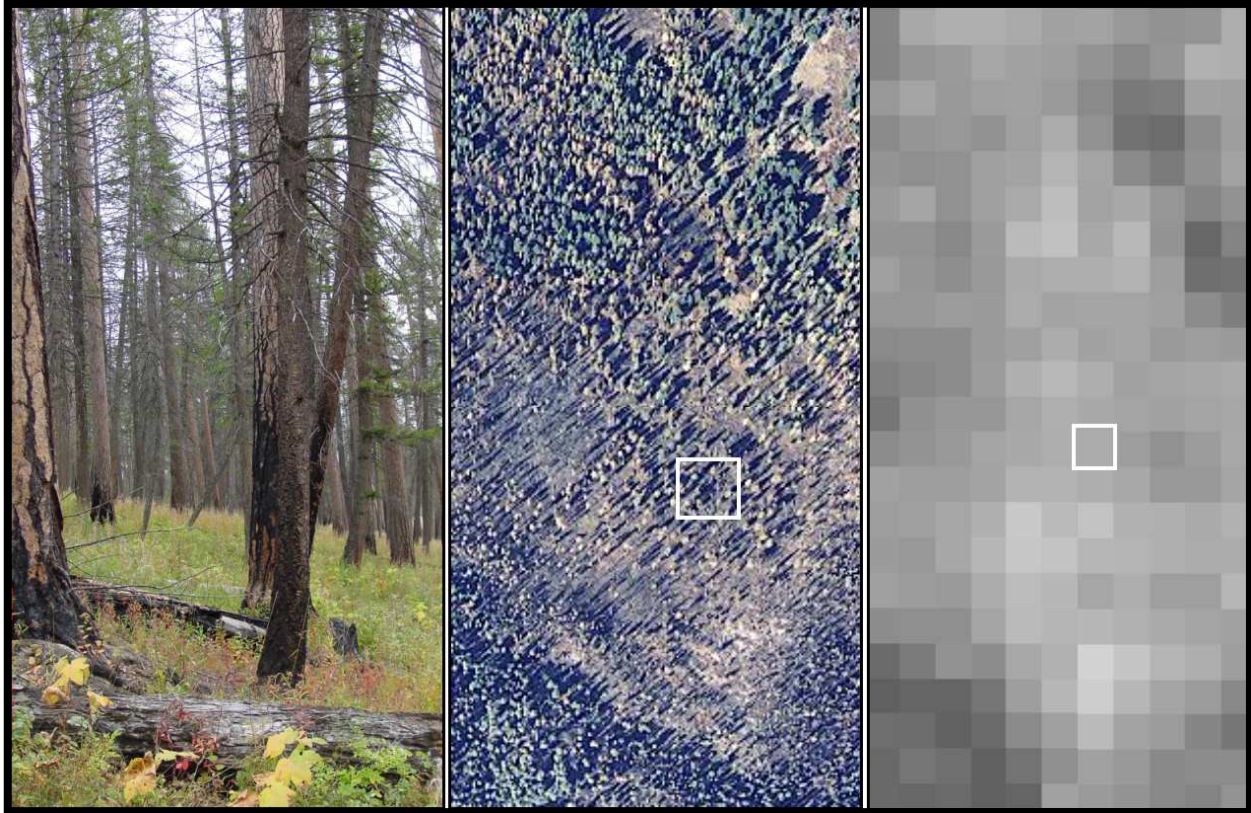
Figure 2. Stepwise aggregation of fire effects occurs as spatial resolution decreases. From left to right, field photo taken about 1 year post-fire; color aerial photo 1 month post-fire; dNBR image using data from 1 month post-fire. White squares, roughly 30x30 m, denote approximate location of the site shown at left.
