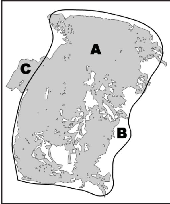
**Figure 3** Percent agreement (A) calculated based on overlap of BLM-mapped polygons and the post-processing polygons from remotely sensed data, with error of commission (B) where it did not burn and error of omission (C) where it did burn but was not mapped as such.
