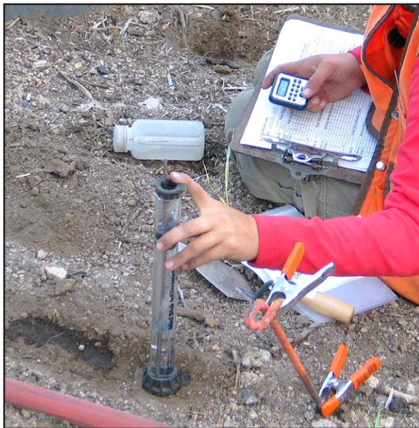
Figure 1: Using a mini-disk infiltrometer to assess soil burn severity and reduced infiltration after a fire.
