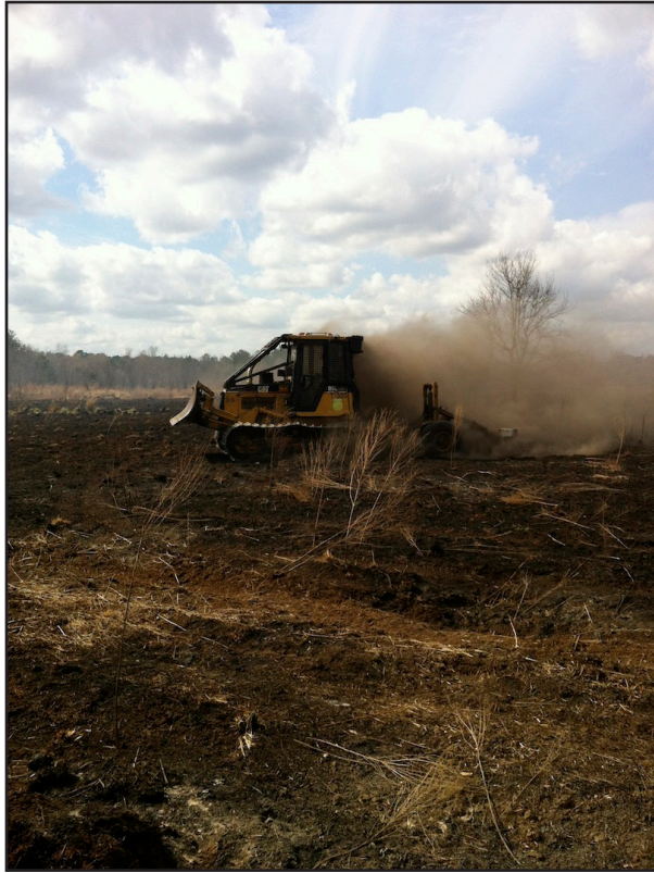
Figure 1. Many passes of this bulldozer were required to cut a fireline to mineral soil through the thick peat at this ground fire in northern Florida, USA.
