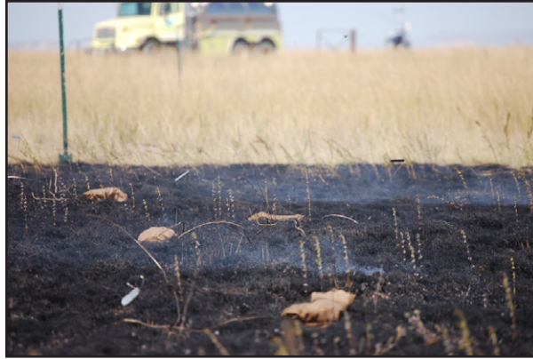
Figure 2. Thermocouples and target plants in a plot burned in October 2011.
