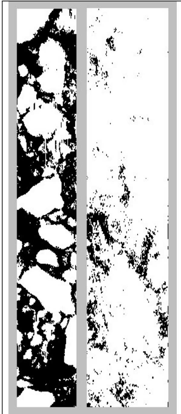
Figure 8. Vertical cross sections (derived from X-ray computed tomography) of Manitou Experimental Forest soil. Black areas of the photographs correspond to soil pore space. The figure on the left corresponds to the upper 0.05 m of the soil from an area unaffected by the slash-pile burn. The figure on the right was obtained from a sample of the soil beneath the slash-pile burn. Cross sections have been calculated from about 200 horizontal slices. The horizontal length of each image is about 2 mm. The pixel resolution is 18 \mu\text{m} .
